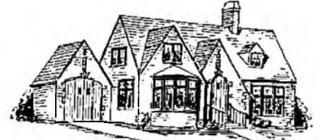
Bad Exterior Design. Complicated gables. Expensive windows. Poor proportions of windows to gables. Too much "architecture" and unnecessary trimming for small home.
