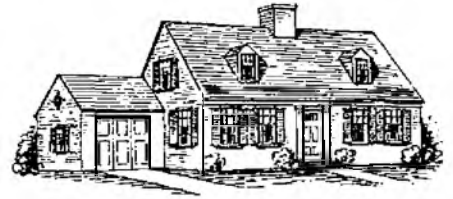
Good Exterior Design. Simple lines left unchanged. Standard millwork planned. Excellent proportions of windows to house. Good basic plan can be built inexpensively.
